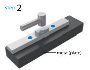
Put the plate on the cap, then pound it into the bolt of rail with rubber hammer vertically.
