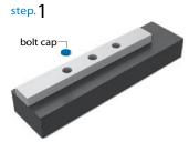
Put the cap into the bolt hole of rail.
